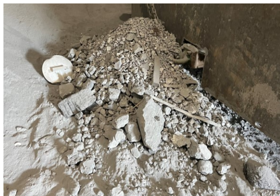
Figure 2. Picture of the debris in contaminated alumina.
